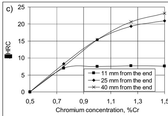
Figure 5: The effect of Cr concentration on hardenability (a - chemical compositions no 1.x, b- chemical compositions no 2.x, c- chemical compositions no 3.x – Table I)
