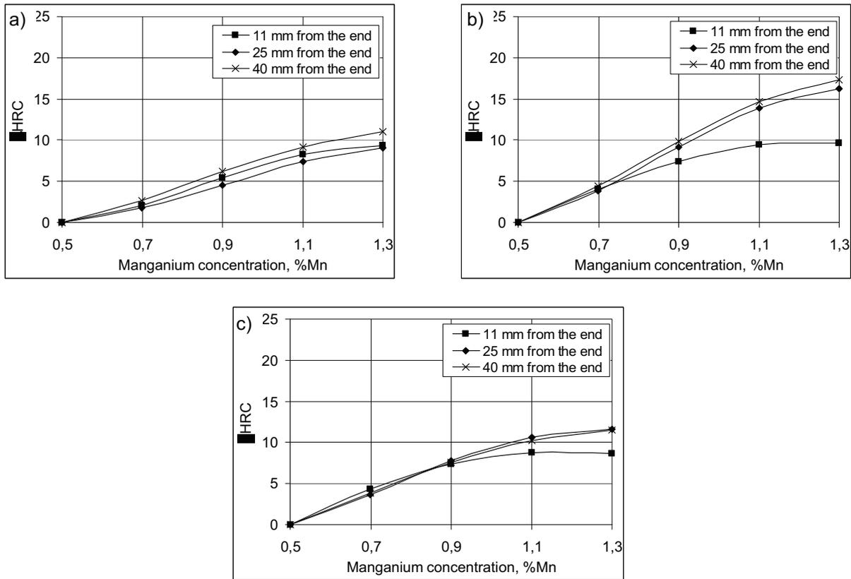
Figure 6: The effect of Mn concentration on hardenability (a - chemical compositions no 4.x, b- chemical compositions no 5.x, c- chemical compositions no 6.x – Table II)
