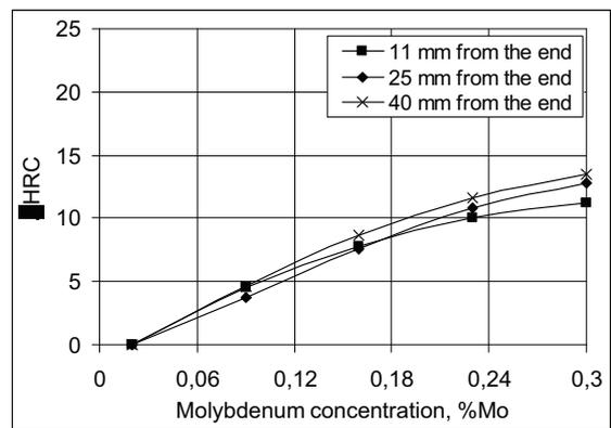
Figure 8: The effect of Mo concentration on hardenability for the chemical compositions no 8.x (Table IV)
