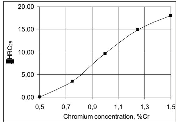
Figure 4: The effect of the Cr concentration on hardness  $H_{25}$  for the 25 mm distance from the Jominy specimen end-quench test
