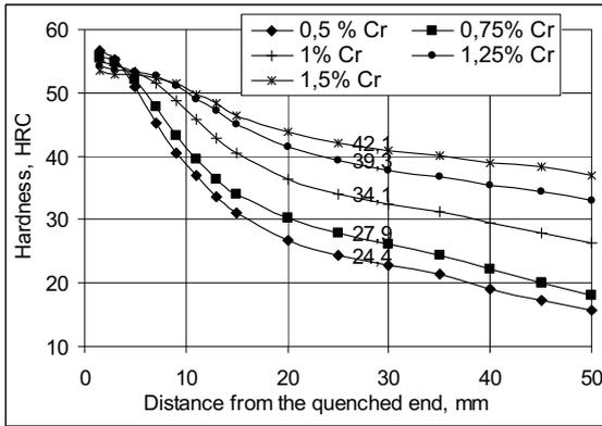
Figure 3: Calculated hardenability curves for the steels with chemical compositions no 1.1 – 1.5
