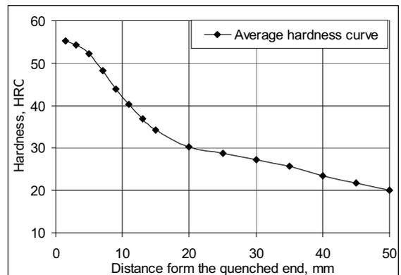
Figure 2: Average hardenability curves for the steel with chemical composition no 1.2.
