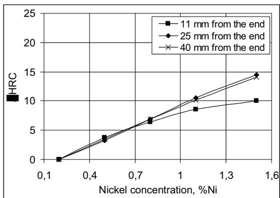
Figure 7: The effect of Ni concentration on hardenability for the chemical compositions no 7.x (Table III)
