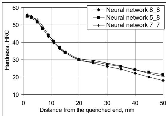
Figure 1: Calculated hardenability curves for the steel with chemical composition no 1.2.
