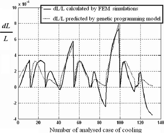
Figure 2. Correspondence between FEM calculated relative changes in length after transformation-free cooling of cylinders made of austenitic steels and predicted by genetic programming model
