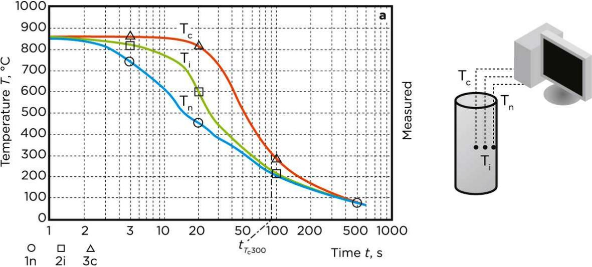
From these recorded cooling curves the following thermodynamic functions are calculated:
