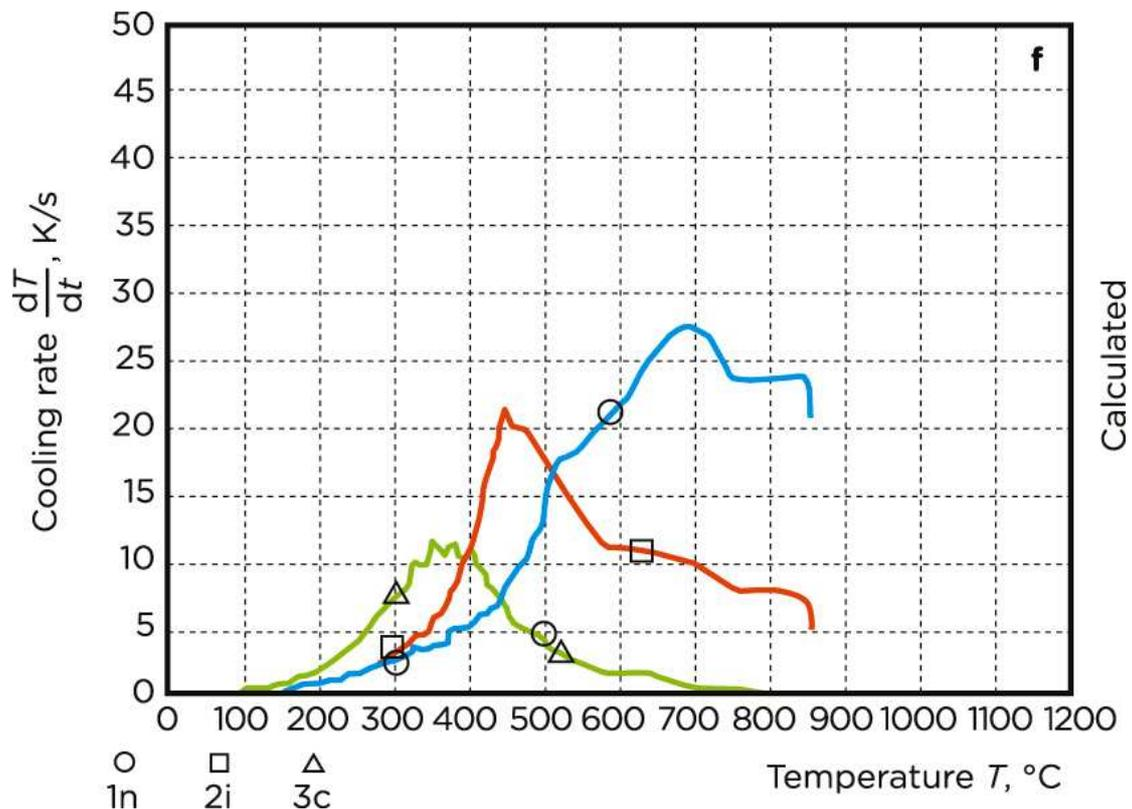
The shown diagrams belong to the case when the Liscic/Nanmac probe was quenched in a mineral oil of 20 °C, without agitation.
